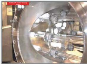
**Ultraviolet disinfection performs best** in waters that contain few UV-absorbing compounds, have low turbidity, and have target organisms that are susceptible to UV disinfection. The water from NSWC meets all of these criteria.
