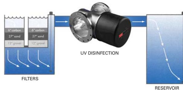
UV disinfection involves pumping filtered water through a reactor containing eight UV light emitting lamps. The UV light inactivates bacteria, pathogens, and viruses found in the filtered water.
